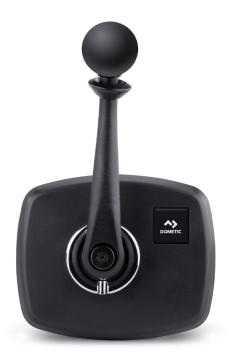
These controls feature superior styling, a compact design, positive lockout with a smooth feel available, allowing for precise throttle control. Dual action design (one lever to control both shift and throttle functions). Waterproof neutral safety switch standard on jet unit (optional on ski model). Uses 3300/33C type cables.
