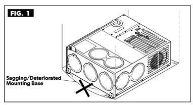
Confirm the Furnace mounting base is not sagging or deteriorating.
